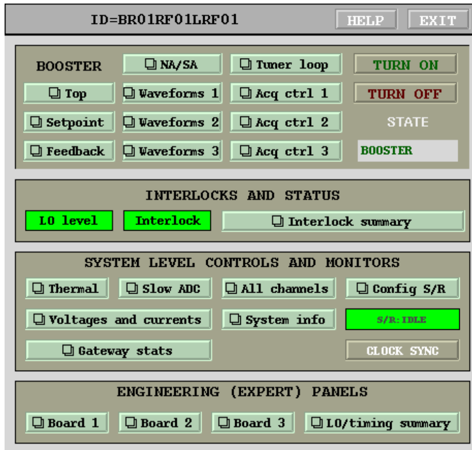
Figure 1: Main LLRF9 control panel.
