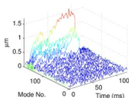
MAX IV 3 GeV Jun1216/163219:  $I_0=40.624\text{mA}$ ,  $D_{\text{samp}}=1$ ,  $\text{ShfGain}=4$ ,  $N_{\text{bun}}=176$ ,
